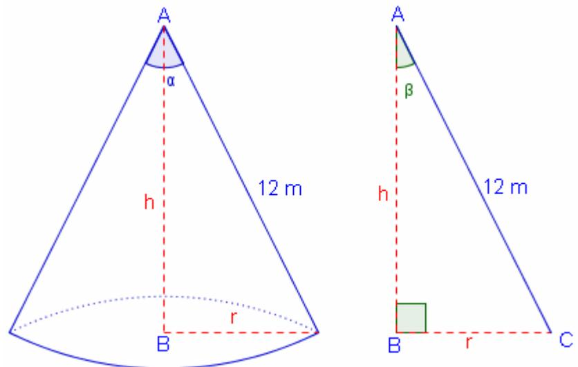
$$\begin{cases} \text{sen} \beta = \frac{BC}{AC} \Leftrightarrow \text{sen} 30^\circ = \frac{r}{12 \text{ m}} \Leftrightarrow r = 12 \text{ m} \cdot \text{sen} 30^\circ = 6 \text{ m} \\ \text{cos} \beta = \frac{AB}{AC} \Leftrightarrow \text{cos} 30^\circ = \frac{h}{12 \text{ m}} \Leftrightarrow h = 12 \text{ m} \cdot \text{cos} 30^\circ = 10,39 \text{ m} \end{cases}$$
