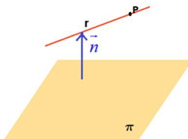
$$d(r, \pi) = d(P, \pi) = \left\{ \begin{array}{l} P(0, 2, 1) \\ \pi : 2x + y - z - 2 = 0 \end{array} \right\} = \frac{|2 \cdot 0 + 2 - 1 - 2|}{\sqrt{2^2 + 1^2 + (-1)^2}} = \frac{1}{\sqrt{6}} = \boxed{0,408 u}$$
