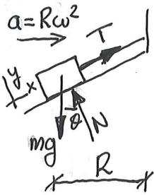
$$\left. \begin{aligned} (2LN)_x: -m g \sin \theta + T &= m R \omega^2 \cos \theta & (1) \\ (2LN)_y: -m g \cos \theta + N &= -m R \omega^2 \sin \theta & (2) \end{aligned} \right\}$$
