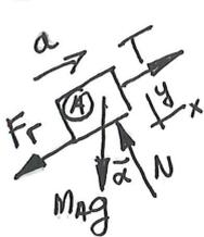
$$\left. \begin{aligned} (2LN)_x^A: -F_r - m_A g \sin \alpha + T &= m_A a & (1) \\ (2LN)_y^A: -m_A g \cos \alpha + N &= 0 & (2) \\ (2LN)_y^B: T - m_B g &= -m_B a & (3) \end{aligned} \right\}$$
