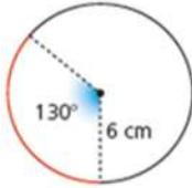
$$l_{\text{arco}} = \frac{2 \cdot \pi \cdot r}{360^\circ} \cdot \hat{A} \Rightarrow l_{\text{arco}} = \frac{2 \cdot 3,14 \cdot 6}{360^\circ} \cdot 130^\circ = 13,61 \Rightarrow l_{\text{arco}} = 13,61 \text{ cm}$$
