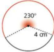
$$l_{\text{arco}} = \frac{2 \cdot \pi \cdot r}{360^\circ} \cdot \hat{A} \Rightarrow l_{\text{arco}} = \frac{2 \cdot 3,14 \cdot 4}{360^\circ} \cdot 230^\circ = 16,05 \Rightarrow l_{\text{arco}} = 16,05 \text{ cm}$$
