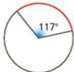
$$l_{\text{arco}} = \frac{2 \cdot \pi \cdot r}{360^\circ} \cdot \hat{A} \Rightarrow l_{\text{arco}} = \frac{2 \cdot 3,14 \cdot 5}{360^\circ} \cdot 117^\circ = 10,21 \Rightarrow l_{\text{arco}} = 10,21 \text{ cm}$$
