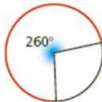
$$l_{\text{arco}} = \frac{2 \cdot \pi \cdot r}{360^\circ} \cdot \hat{A} \Rightarrow l_{\text{arco}} = \frac{2 \cdot 3,14 \cdot 5}{360^\circ} \cdot 260^\circ = 22,68 \Rightarrow l_{\text{arco}} = 22,68 \text{ cm}$$
