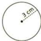
$$A_{\text{círculo}} = \pi \cdot r^2 \Rightarrow A_{\text{círculo}} = 3,14 \cdot 3^2 = 28,26 \Rightarrow A_{\text{círculo}} = 28,26 \text{ cm}^2$$
