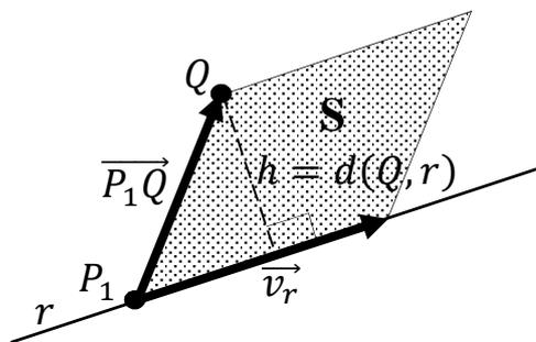
$$\left. \begin{aligned} S &= |\vec{v}_r \wedge \overrightarrow{P_1Q}| \\ S &= |\vec{v}_r| \cdot h \end{aligned} \right\} \Rightarrow |\vec{v}_r \wedge \overrightarrow{P_1Q}| = |\vec{v}_r| \cdot h \Rightarrow$$
