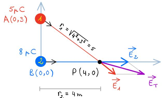
$$\vec{E}_1 = k \frac{Q_1}{r_1^2} \vec{u}_1 = 9 \cdot 10^9 \cdot \frac{5 \cdot 10^{-9}}{5^2} \left( \frac{4}{5} \vec{i} - \frac{3}{5} \vec{j} \right) \frac{\text{N}}{\text{C}} = \frac{36}{25} \vec{i} - \frac{27}{25} \vec{j} = 1,44 \vec{i} - 1,08 \vec{j} \frac{\text{N}}{\text{C}}$$
