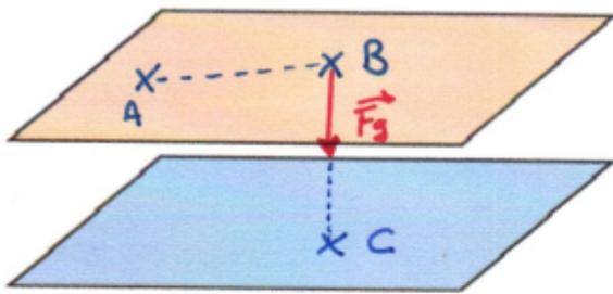
$$\begin{aligned} W_{B \rightarrow C} &= \int_B^C \vec{F} \cdot d\vec{r} = -\Delta E_p = \\ &= -(E_{pC} - E_{pB}) = \\ &= -(-1000 + 800) = +200 \text{ J} \end{aligned}$$
