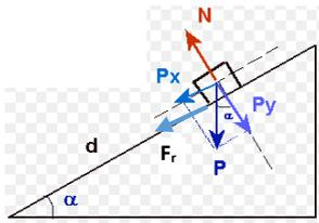
$$P_x = P \sin \alpha = m \cdot 10 \sin 30 = 5\text{m} \quad P_y = P \cos \alpha = m \cdot 10 \cos 30 = 8,7\text{m} \quad F_r = \mu N = 0,1 P_y = 0,87\text{N}$$
