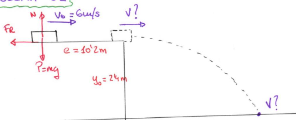
$$P = mg; \quad N = P = mg; \quad F_Q = \mu \cdot N = 0.1 \cdot mg$$
