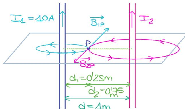
módulos:  $B_{1P} = \frac{\mu_0 I_1}{2\pi d_1}$        $B_{2P} = \frac{\mu_0 I_2}{2\pi d_2}$
