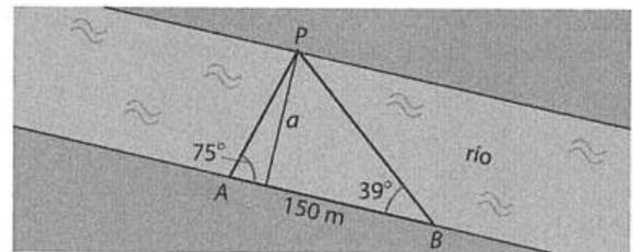
$$\begin{cases} \text{tg } 75^\circ = \frac{a}{(150 - x)} \\ \text{tg } 39^\circ = \frac{a}{x} \end{cases} \Rightarrow a = 99,81 \text{ m}$$
