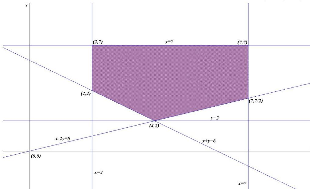
$$\begin{aligned} z(4, 2) &= 14000 \\ z(2, 4) &= 16000 \\ z(2, 7) &= 25000 \\ z(7, 7) &= 35000 \\ z(7, 7/2) &= 24500 \end{aligned}$$
