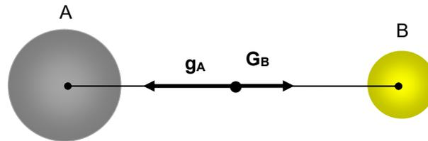
$$\left. \begin{array}{l} g_A = G \frac{M_A}{r^2} \\ g_B = G \frac{M_B}{r^2} \end{array} \right\} g_{\text{Tot}} = g_A - g_B = \frac{G}{r^2} (M_A - M_B) = \frac{6,67 \cdot 10^{-11} \frac{\text{N m}^2}{\text{kg}^2}}{8^2 \text{ m}^2} (5000 - 3000) \text{ kg} = 8,34 \cdot 10^{-9} \frac{\text{N}}{\text{kg}}$$
