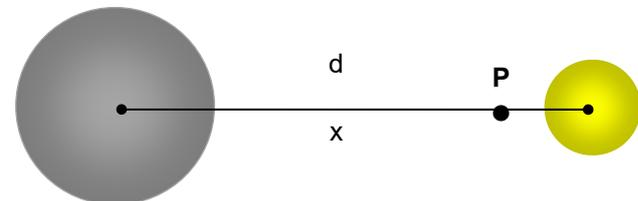
$$\left. \begin{aligned} F_T &= G \frac{m M_T}{x^2} \\ F_L &= G \frac{m M_L}{(d-x)^2} \end{aligned} \right\} G \frac{M_T}{x^2} = G \frac{M_L}{(d-x)^2}; \left( \frac{d-x}{x} \right)^2 = \frac{M_L}{M_T}; \frac{d-x}{x} = \sqrt{\frac{M_L}{M_T}} = \sqrt{\frac{1}{81}} = \frac{1}{9}$$
