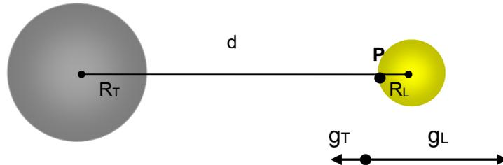
$$\left. \begin{aligned} g_T &= G \frac{M_T}{r^2} \\ g_L &= G \frac{M_L}{R_L^2} \end{aligned} \right\} \begin{aligned} g_T &= \frac{M_T R_L^2}{M_L r^2} = \frac{5,97 \cdot 10^{24} \text{ kg} (1,7 \cdot 10^6)^2 \text{ m}^2}{7,35 \cdot 10^{22} \text{ kg} (3,8 \cdot 10^8)^2 \text{ m}^2}; \quad \boxed{g_T = 1,6 \cdot 10^{-3} g_L} \end{aligned}$$
