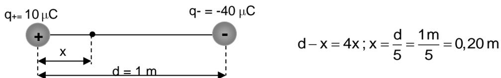
$$d - x = 4x ; x = \frac{d}{5} = \frac{1 \text{ m}}{5} = 0,20 \text{ m}$$
