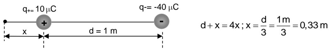
$$d + x = 4x ; x = \frac{d}{3} = \frac{1 \text{ m}}{3} = 0,33 \text{ m}$$
