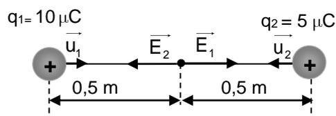
$$\vec{E}_1 = \left( K \frac{q_1}{r_1^2} \right) \vec{u}_1 = \left( 9 \cdot 10^9 \frac{\text{N m}^2}{\text{C}^2} \frac{10 \cdot 10^{-6} \text{ C}}{(0,5)^2 \text{ m}^2} \right) \vec{i} = (3,6 \cdot 10^5) \vec{i} \left( \frac{\text{N}}{\text{C}} \right)$$
