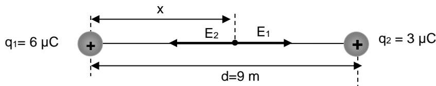
$$\left. \begin{array}{l} E_1 = K \frac{q_1}{x^2} \\ E_2 = K \frac{q_2}{(d-x)^2} \end{array} \right\} E_1 = E_2; K \frac{q_1}{x^2} = K \frac{q_2}{(d-x)^2}; \frac{x^2}{(d-x)^2} = \frac{q_1}{q_2}; \frac{x}{d-x} = \sqrt{\frac{6 \cdot 10^{-6} \cancel{\text{C}}}{3 \cdot 10^{-6} \cancel{\text{C}}}}; x = 5,27 \text{ m}$$
