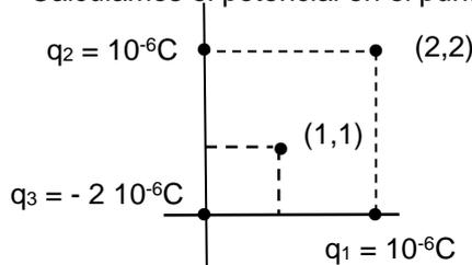
$$V_1 = V_2 = K \frac{q}{r} = 9 \cdot 10^9 \frac{\text{N} \cdot \text{m}^2}{\text{C}^2} \frac{10^{-6} \text{ C}}{\sqrt{2} \text{ m}} = 6364 \left( \frac{\text{J}}{\text{C}} \right) (\text{V})$$
