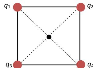
$$\begin{aligned} E_{PT} &= \sum_{i \neq j} k \cdot \left( \frac{q_i \cdot q_j}{r_{ij}} \right) = \\ &= k \cdot \left[ \left( \frac{q_1 \cdot q_2}{r_{12}} \right) + \left( \frac{q_1 \cdot q_3}{r_{13}} \right) + \left( \frac{q_1 \cdot q_4}{r_{14}} \right) + \left( \frac{q_2 \cdot q_3}{r_{23}} \right) + \left( \frac{q_2 \cdot q_4}{r_{24}} \right) + \left( \frac{q_3 \cdot q_4}{r_{34}} \right) \right] \end{aligned}$$
