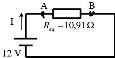
$$\frac{1}{R_{eq}} = \frac{1}{R_1} + \frac{1}{R_2} + \frac{1}{R_3} = \frac{R_2 \cdot R_3 + R_1 \cdot R_3 + R_1 \cdot R_2}{R_1 \cdot R_2 \cdot R_3}$$
