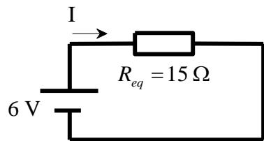
$$R_{eq} = R_1 + R_2 = 5 + 10 = 15 \Omega$$
