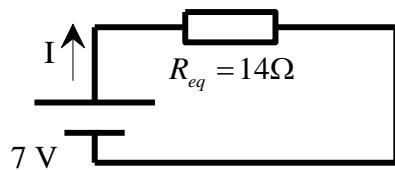
$$R_{eq} = R_1 + R_2 + R_3 = 3 + 6 + 5 = 14 \Omega$$
