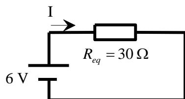
$$R_{eq} = R_1 + R_2 = 15 + 15 = 30 \Omega$$
