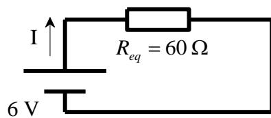
$$R_{eq} = R_1 + R_2 + R_3 = 15 + 15 + 30 = 60 \Omega$$
