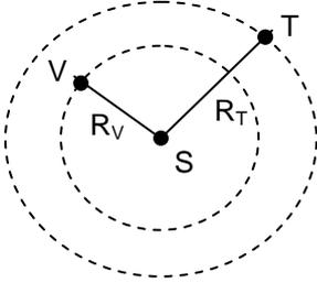
$$\left. \begin{array}{l} R_T = c t_T \\ R_V = c t_V \end{array} \right\} \Rightarrow \frac{R_V}{R_T} = \frac{t_V}{t_T} \rightarrow \frac{R_V}{R_T} = \frac{6.01}{8.31} = 0.723$$
