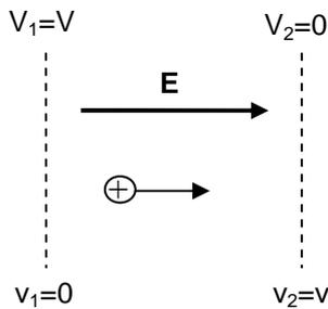
$$E_1 = E_2 \Leftrightarrow 0 + q V_1 = \frac{1}{2} m v_2^2 + q V_2 \Leftrightarrow$$
