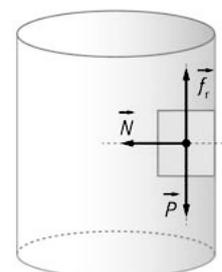
$$v = \omega R \Rightarrow \omega = \frac{v}{R} = \frac{(7,0 \text{ ms}^{-1})}{(4 \text{ m})} = 1,75 \text{ rad s}^{-1} = \left( \frac{1,75 \text{ rad}}{1 \text{ s}} \right) \left( \frac{60 \text{ s}}{1 \text{ min}} \right) \left( \frac{1 \text{ vuelta}}{2\pi \text{ rad}} \right) = 17 \text{ rpm}$$
