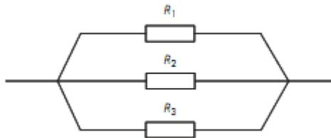
$$\frac{1}{R_{eq}} = \frac{1}{R_1} + \frac{1}{R_2} + \frac{1}{R_3} + \dots$$
