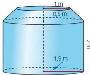
$$V_{\text{Figura}} = V_{\text{Cilindro}} + V_{\text{Tronco de cono}}$$
