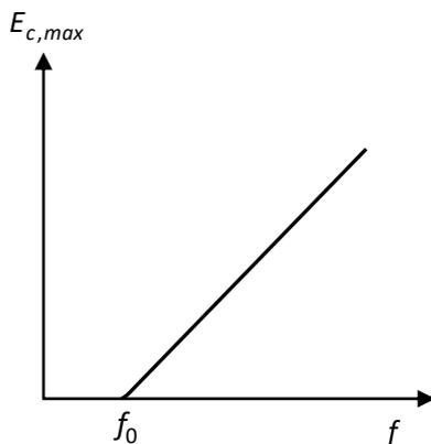
$$\left. \begin{array}{l} hf = W_{ext} + E_{c,max} \\ W_{ext} = hf_0 \end{array} \right\} \Rightarrow hf = hf_0 + E_{c,max} \Rightarrow E_{c,max} = hf - hf_0 \text{ (donde } hf_0 = \text{cte)}$$
