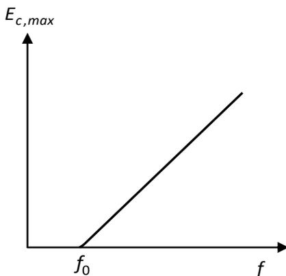
$$\left. \begin{array}{l} E = W_{ext} + E_{c,max} \\ W_{ext} = hf_0 \\ E = hf \end{array} \right\} \Rightarrow E_{c,max} = hf - hf_0$$
