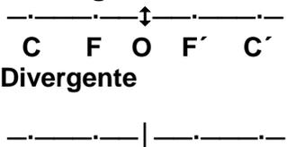
Divergente | <ul style="list-style-type: none"> <li>▪ CENTROS DE CURVATURA (C Y C')</li> <li>▪ EJE PRINCIPAL (CC')</li> <li>▪ CENTRO ÓPTICO O CENTRO DE FIGURA (O)</li> <li>▪ FOCO IMAGEN (F')</li> <li>▪ FOCO OBJETO (F)</li> <li>▪ DISTANCIA FOCAL IMAGEN <math>f' = OF'</math></li> </ul> |
