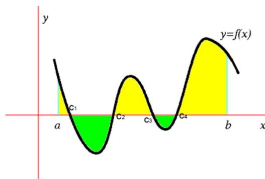
$$Area = +\int_a^{c_1} f(x)dx - \int_{c_1}^{c_2} f(x)dx + \int_{c_2}^{c_3} f(x)dx - \int_{c_3}^{c_4} f(x)dx + \int_{c_4}^b f(x)dx$$
