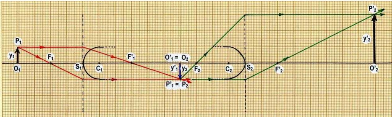
Dioptrio 1°:  $r_1 = S_1C_1 = 5 \text{ cm}$      $n_1 = 1$      $n'_1 = 1,5$      $s_1 = S_1O_1 = -20 \text{ cm}$
